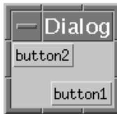
FIGURE 2-5 Spring Layout: Button1 placed 30 pixels from the North and West edges of the Spring
